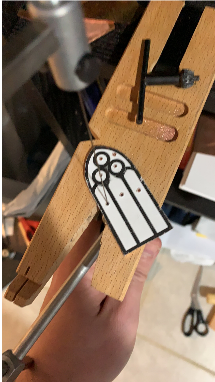
Figure 3: Saw threaded through copper to remove negative space.
