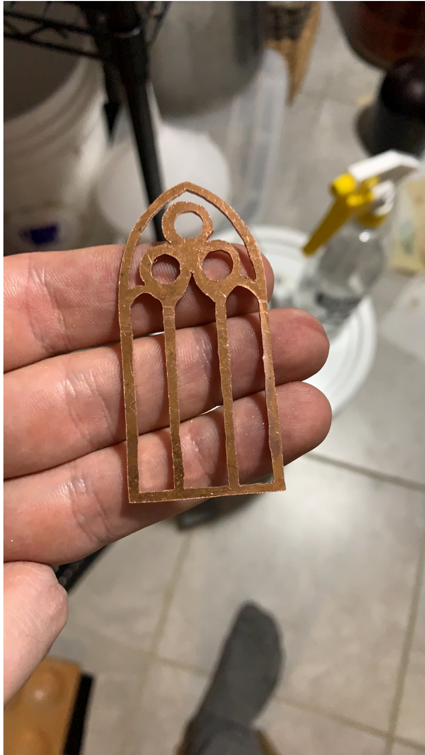
Figure 4: Merode Cup window fully cut out and ready for Plique-a-Jour. 1
