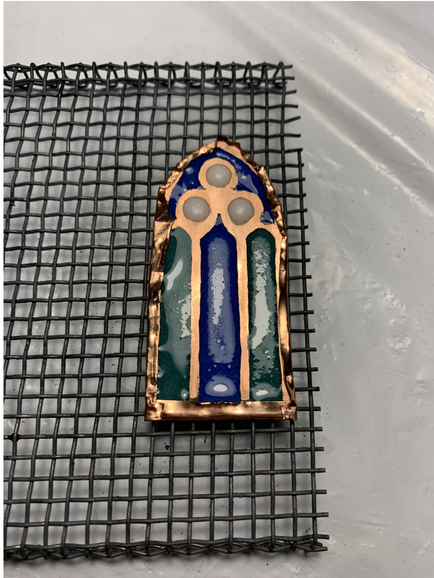
Figure 6: Negative space filled with wet enamel before drying and firing in the kiln at 1450 F. This is the first run through the kiln.
