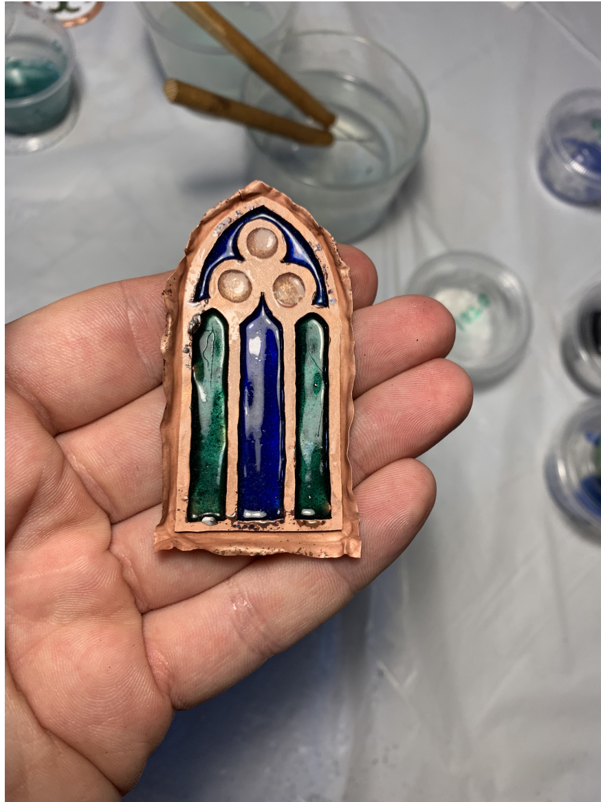
Figure 7: PaJ window after the first run through the kiln. Notice how much lower the enamel has become due to fusing.
